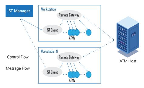
The above diagram shows the architecture of the stress test module.
